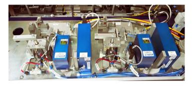
TQC also provided a leak test bench for leak testing of variant pumps. This system allows operators to load and unload parts that have flying leads and other variations.
